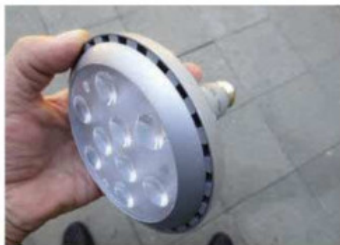
This floodlight has multiple LEDs inside, and screws into a household light socket.
